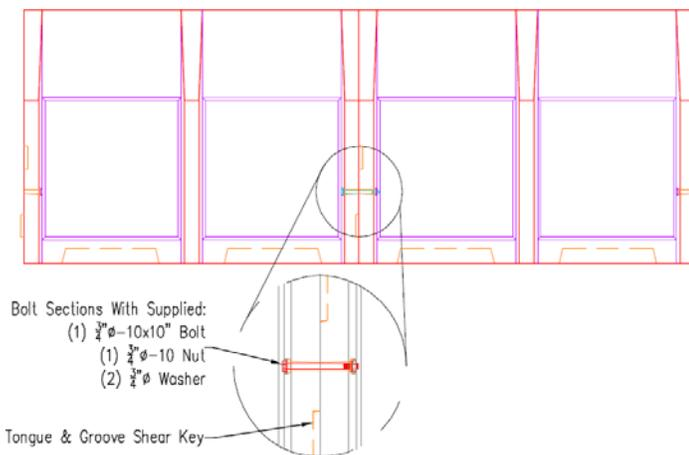
**Figure 3 Typical bolt connection**
